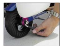
2) With Quick Release Axle opened and loosened, rotate purple engine protection washer (EPW) down, away from rear gas tank support stud.
